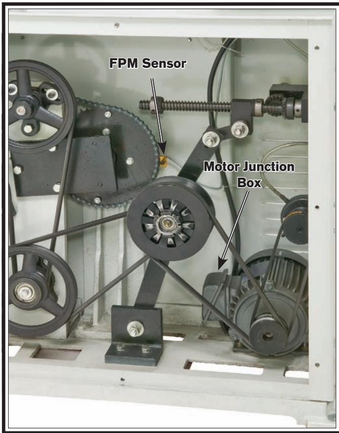
Figure 53. Motor and FPM sensor.
